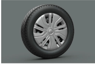
175/65R14 tires + 14-inch steel wheels with cover
