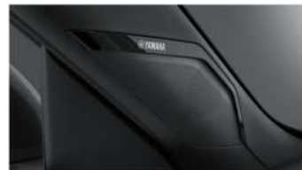
Front dome tweeter on A pillar
